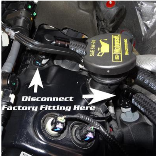
Disconnect the factory vent line by releasing the tab on each end and pull up.
