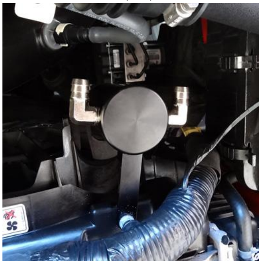
Disconnect the factory vent line by releasing the tab on each end and pull up.
