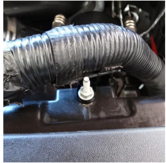
Remove this nut on the top of the fan shroud.
