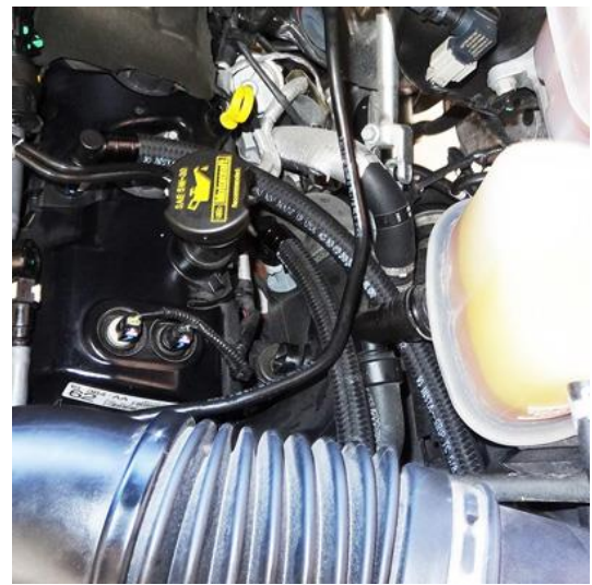
Install the factory Ford fittings on the provided hoses. Connect the inlet side of the can to the valve cover and the outlet side of the can to the intake.
